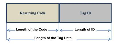
Fig. 2: The structure of the tag data.
