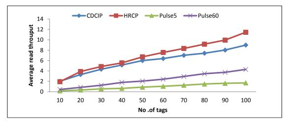
Fig 4: system average read throughput CDCIP and PULSE and HRCP in state 60 reader.
